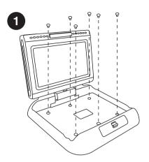
Disassemble the metal support bracket from the unit by unscrewing the six screws.
